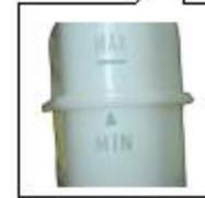
When engine is cold, coolant shall be within MAX and MIN scale on expansion tank. Level rises with engine temperature increasing and falls with engine cooling. If coolant level is under MIN scale, add anti-freezing mixture of 50% water and 50% glycol to improve anti-freezing and antiseptis performance.
